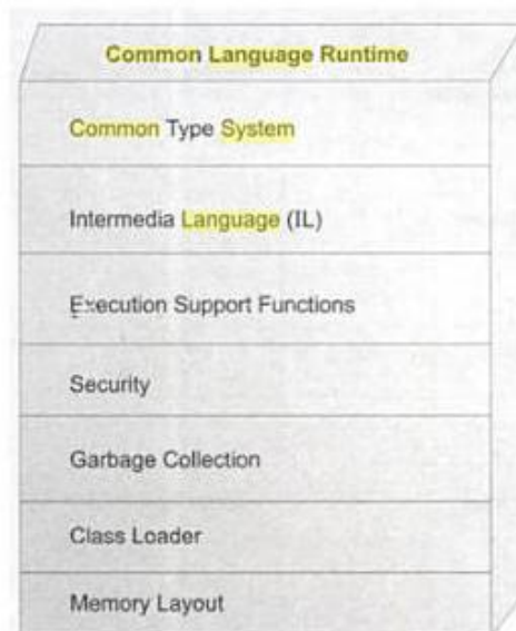
Figure 2.4 Architecture of .NET Framework
