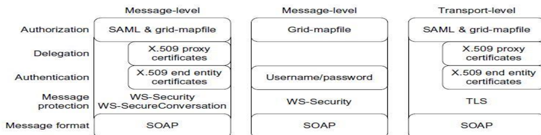
GSI functional layers at the message and transport levels.
