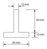
4. An I-section beam having the cross-sectional dimensions shown in Fig. carries a vertical shear load of 80 kN. Calculate and sketch the distribution of vertical shear stress across the beam section and determine the percentage of the total shear load carried by the web.
