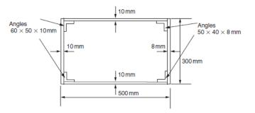
1. Explain how Needham's method is used to determine the crippling stress for a thin-walled channel section. Using the same determine the crippling stress for the section shown in Figure. Compressive yield stress is 250 MPa and modulus of elasticity is 70 GPa. Thickness is 3 mm throughout
