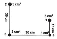
3. A thin-walled, cantilever beam of unsymmetrical cross-section supports shear loads at its free end as shown in Fig. P.16.2. Calculate the value of direct stress at the extremity of the lower flange (point A) at a section half-way along the beam if the position of the shear loads is such that no twisting of the beam occurs.
