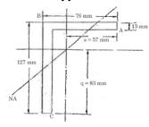
2. Determine the bending stresses developed in the idealized section shown in Figure 16(a). The section is subjected to bending moments with respect to centroidal axes Xand Y and they are MX= 5 kN-m and MY= 1 kN-m.
