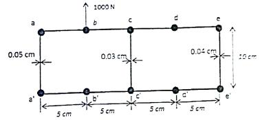
1. A thin-walled two-cell beam with the singly symmetrical cross-section shown in Fig. P.26.2 is built-in at one end where the torque is 11 000 Nm. Assuming the cross-section remains undistorted by the loading, determine the distribution of shear flow and the position of the centre of twist at the built-in end. The shear modulus *G* is the same for all walls.
