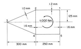
2. Idealize the box section shown in Fig. P.20.1 into an arrangement of direct stress carrying booms positioned at the four corners and panels which are assumed to carry only shear stresses. Hence determine the distance of the shear centre from the left-hand web.
