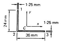
2. Find the shear flow distribution and locate the shear center location for the section shown in figure. For a vertical shear load of Sy = 50kN acting through shear center. Area of all stringers is same which is equal to 2cm<sup>2</sup>
