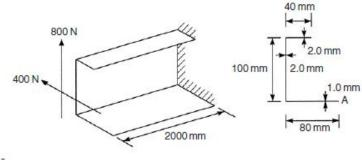
1. The centroid location of the thin-walled angle section given in Figure 5 is (11.274mm, 5.2 mm) from corner 2. The section is subject to vertical shear of 300 N. Determine expressions for the resulting shear flow. Plot the shear flow pattern. Wall thickness is uniform and equal to 1.25 mm.
