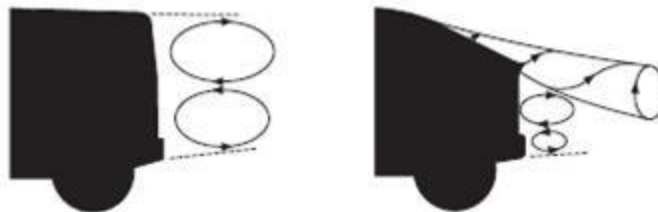
(a) 'Squareback' large scale flow separation. (b) 'Hatchback/Fastback' vortex generation
